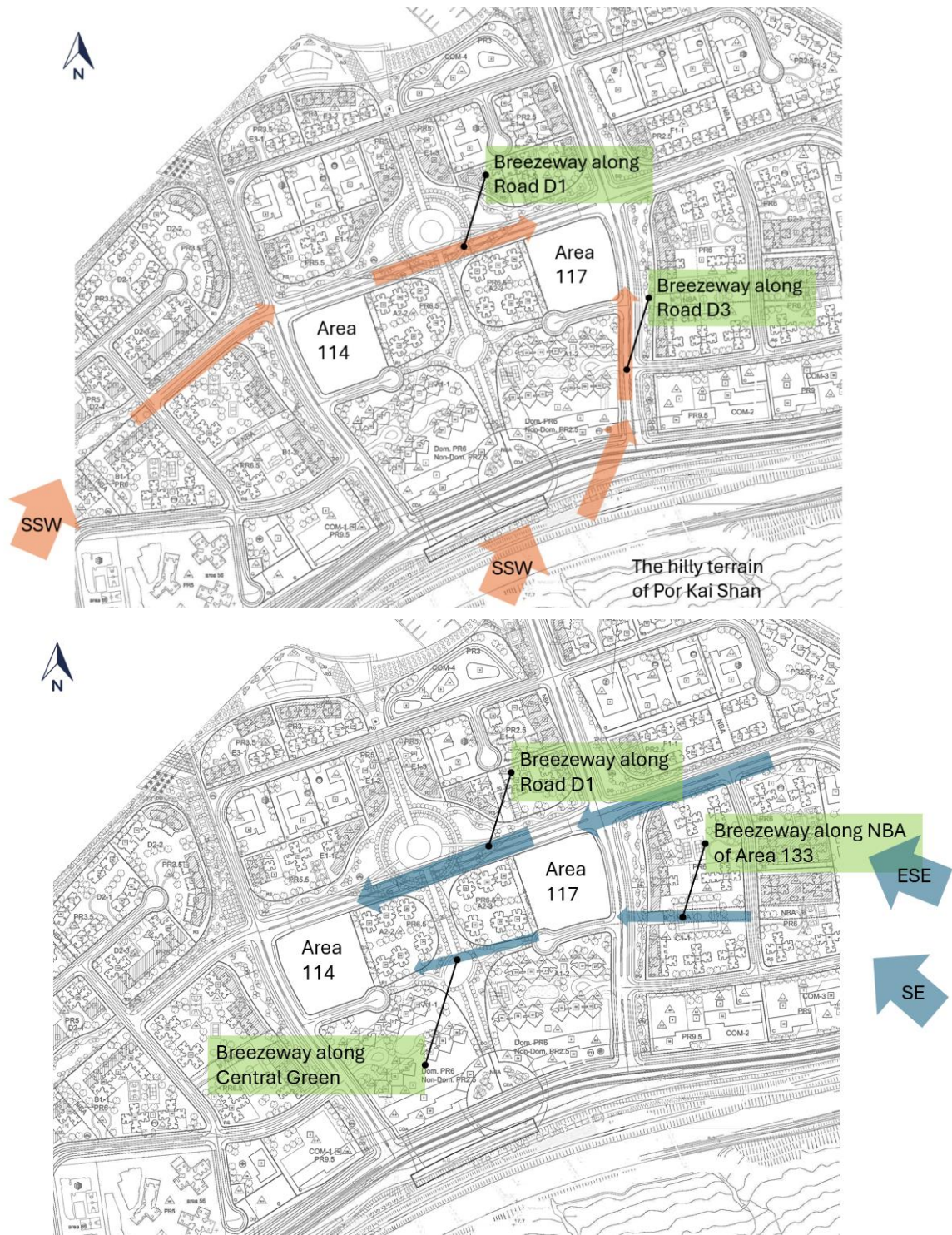
Figure 5 – Expected Wind Flow Pattern under Summer Prevailing SSW Wind (Top), and ESE and SE Wind (Bottom)
